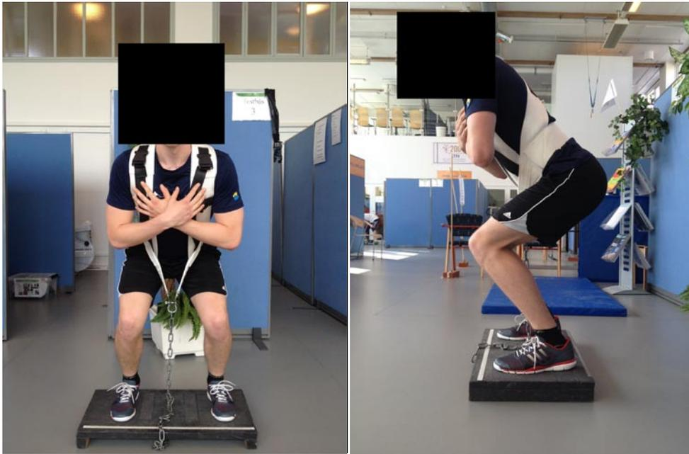
**Figure 2.** The apparatus and participant position used when performing the conditioning contraction. This was also used to determine the participant's RFD and peak power when performing the  $ISO_{max}$  at the familiarization (FAM) session and experimental (EXP) session.
