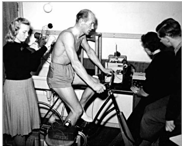
**Fig. 4.** The cycle ergometer was developed at GIH
